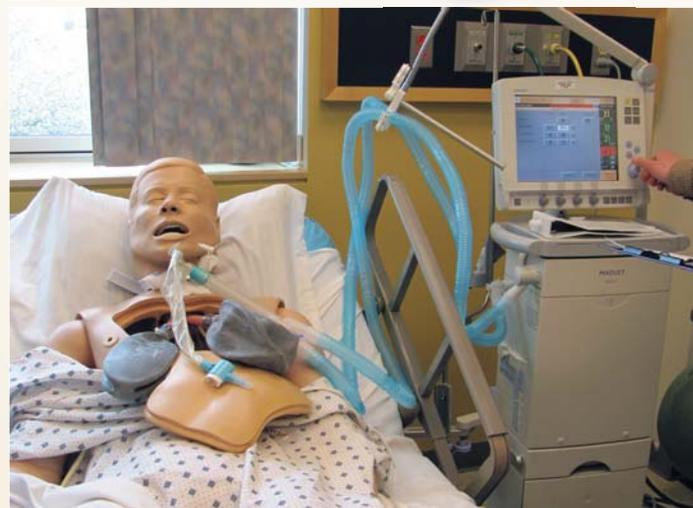
Instructor at the Northern Virginia Community College (NVCC) uses a simulation mannequin to test the performance of the Passy-Muir Valve in-line with a ventilator.
